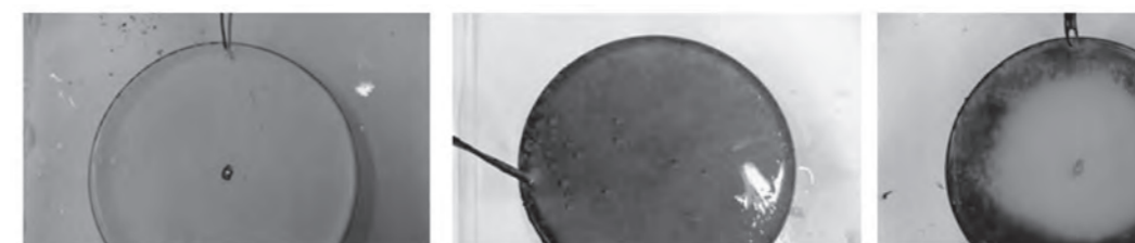
Figure 1. Three test samples. Left: sample before test. Middle: reference sample without UV light emission, after 4 weeks in water. Right: sample with UV light emission after same time period.
