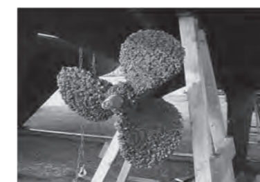
Removal of a copper coated propeller from the electrolytic bath
