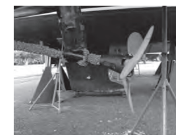
Photograph of a copper-coated propeller after three summer month deployment at the west-coast. Note the absence of barnacle growth at the propeller blades. Also note the presence of barnacles at the propeller axis.
