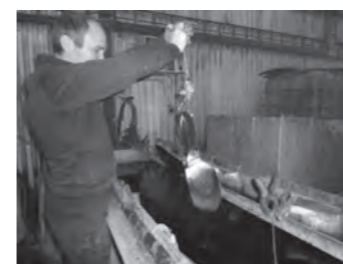
Typical appearance of a Yacht propeller at the west coast of Sweden after three summer month. Note the dense growth of barnacles at the propeller-blades.
