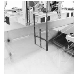
Figure 3. The frame with model attached to towing carriage in the hydrodynamics laboratory at the United States Naval Academy. Forces on the frame/model at different towing speeds were measured.
