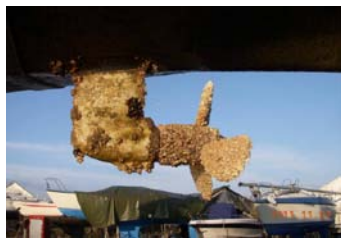
Figure. Left: Barnacle covered propeller Right: The push force (kN) of the type propeller has been plotted against the applied axis power (kW) of the propeller..
