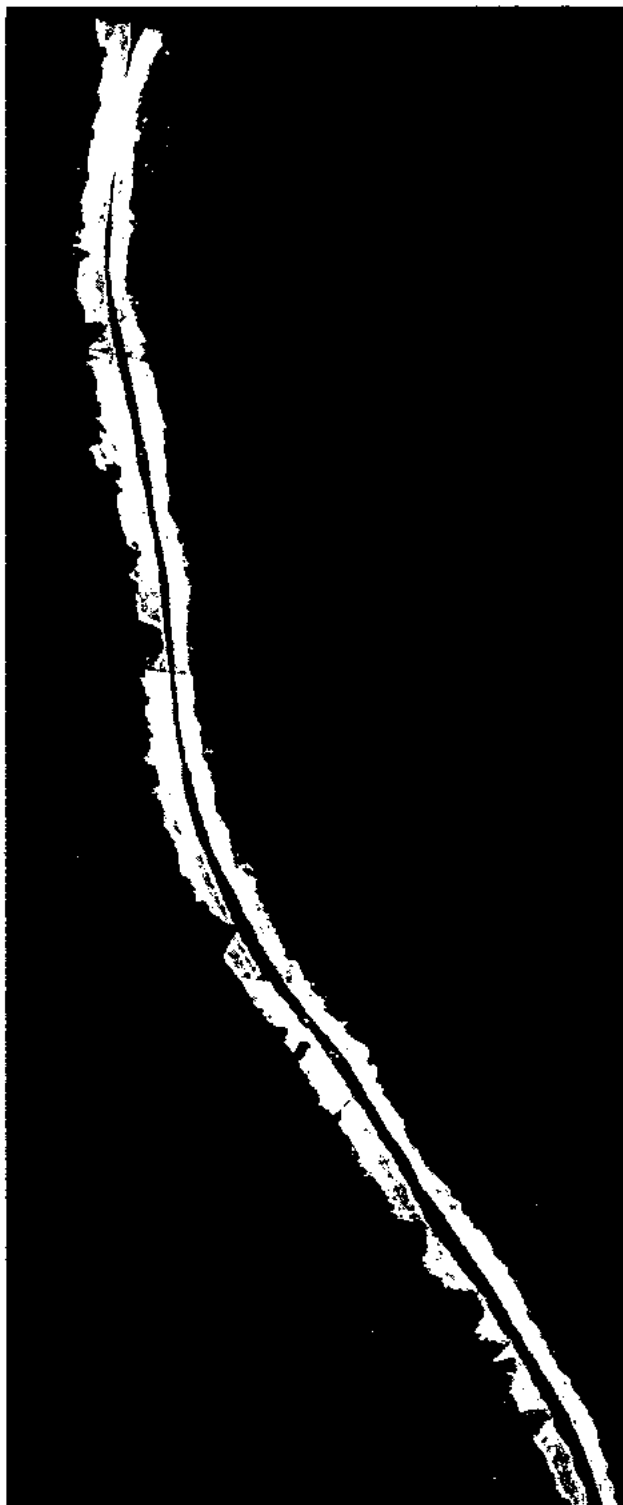
FIG. 9. — Cross-sections of two paint systems, both aged on the raft. Both antifouling paints are of the continuous contact type. It is clear that the layer of \text{Cu}_2\text{O} remaining varies greatly in thickness; in the left-hand illustration the \text{Cu}_2\text{O} has disappeared completely at one spot.
