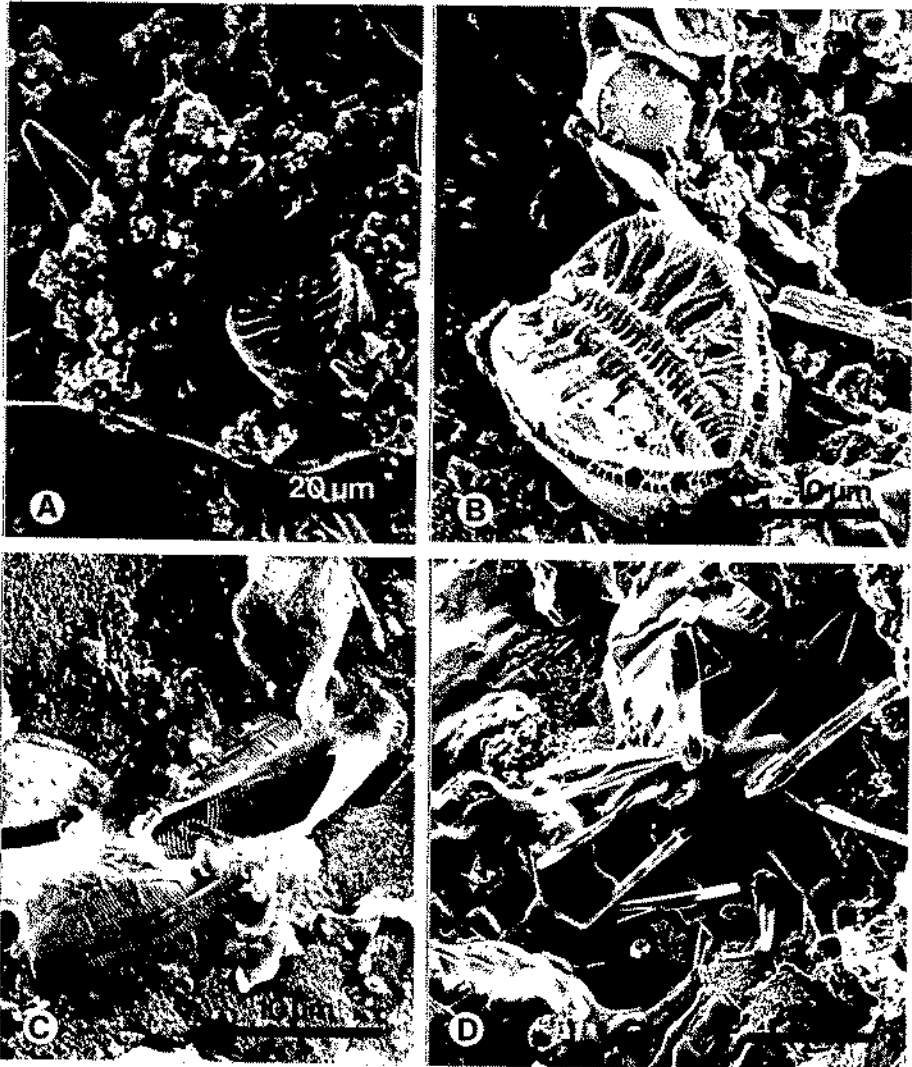
Plate 1 - Microfouling on steel. A. Diatoms (D) trapped in rust product. B. Diatoms (M = Melosira , C = Campilyodiscus sp.) trapped by carbonate scale on protected steel. C. Diatom remains becoming buried in carbonate scale. D. Benthic diatoms producing copious mucilage over carbonate scale. All after 100 days immersion.
